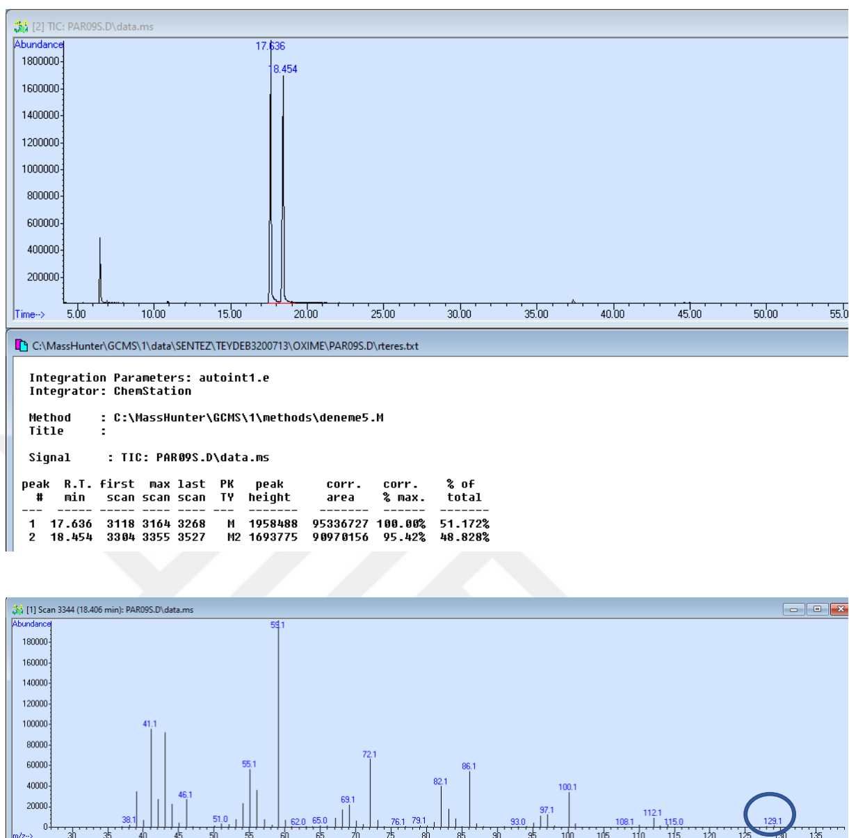
Figure 6-24-GC-MS spectrum of 2.2h
