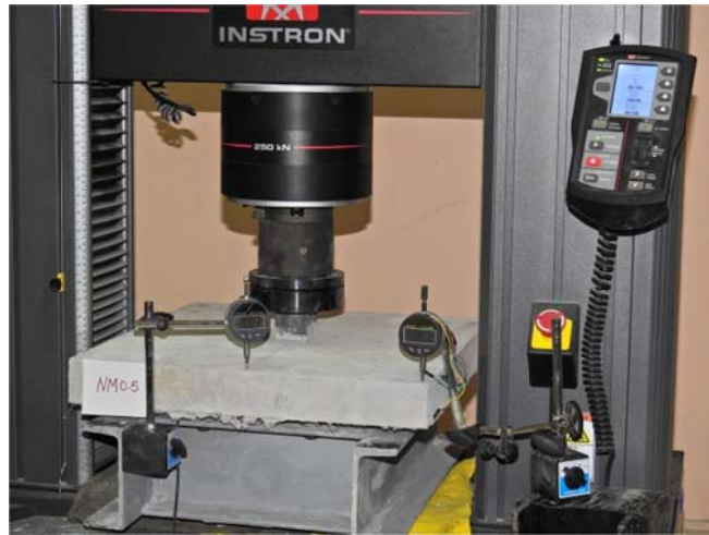
Figure 3.20 Test configuration of slab specimens
