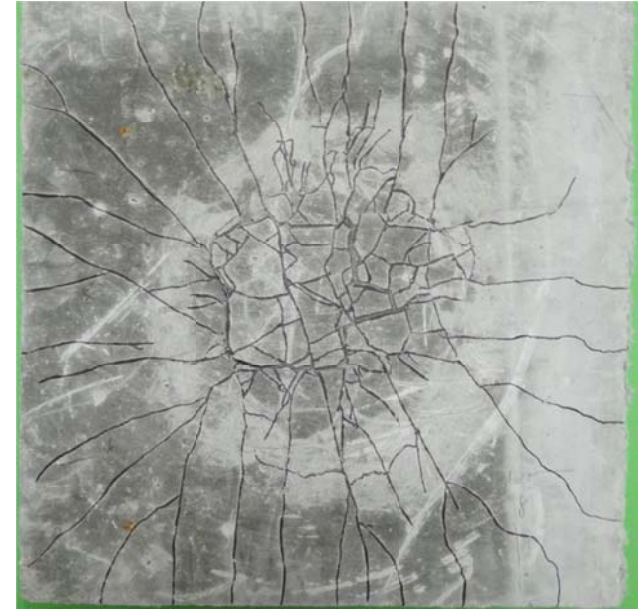
Specimen code; PP12 P_u = 59.23 \text{ kN} f'_c = 31.51 \text{ MPa} \rho = 1.2 \% V_f = 2 \% of PP12 mm-ECC (RC slab)
