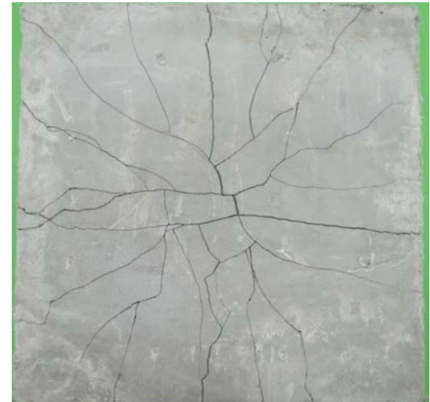
Specimen code; NM2 P_u = 23.5 \text{ kN} f'_c = 36.06 \text{ MPa} \rho = 0.0 \% V_f = 2 \% of NMECC
