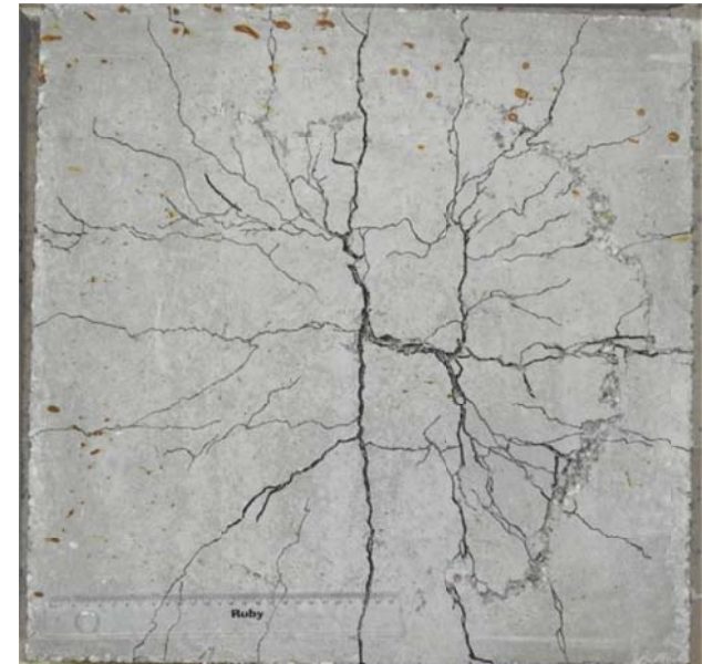
Specimen code; SF1.5 P_u = 92.83 \text{ kN} f'_c = 80.88 \text{ MPa} \rho = 1.1 \% V_f = 1.5 \% of SFRC
