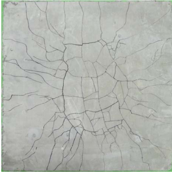
Specimen code; NM0.5R P_u = 59.75 \text{ kN} f'_c = 37.94 \text{ MPa} \rho = 1.1 \% V_f = 0.5 \% of NMECC
