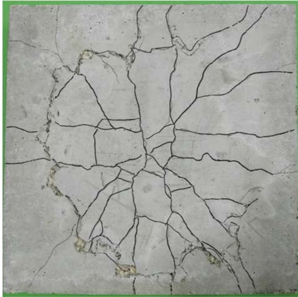
Specimen code; P50 P_u = 51.31 \text{ kN} f'_c = 43.20 \text{ MPa} h = 50 \text{ mm} Normal concrete
