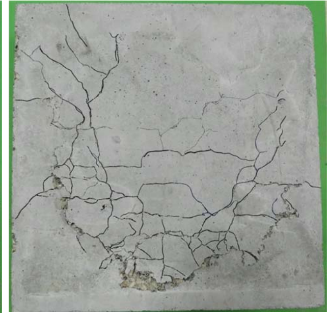
Specimen code; P80 P_u = 120.71 \text{ kN} f'_c = 43.20 \text{ MPa} h = 80 \text{ mm} Normal concrete
