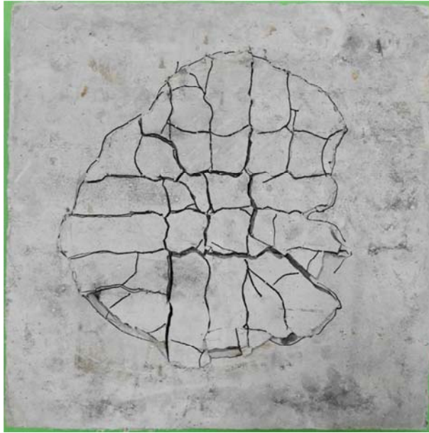
Specimen code; PV6 P_u = 92.42 \text{ kN} f'_c = 43.18 \text{ MPa} \rho = 1.2 \% V_f = 2 \% of PVA6 mm-ECC (RC slab)
