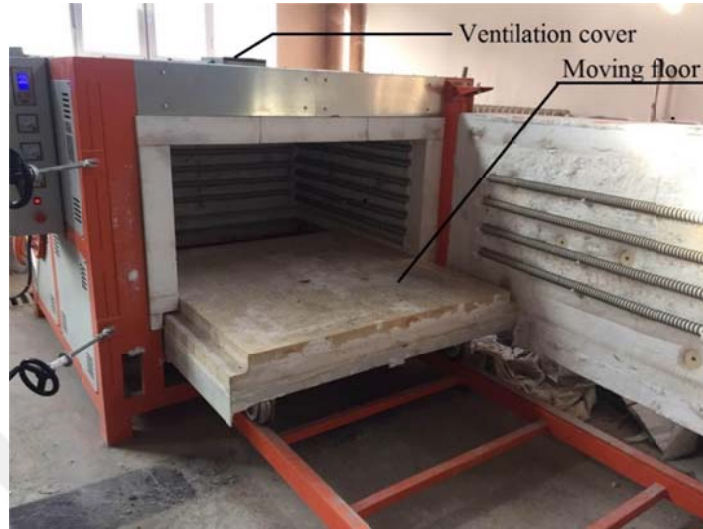
Figure 3.18 Furnace of 1360×1300×620 mm
