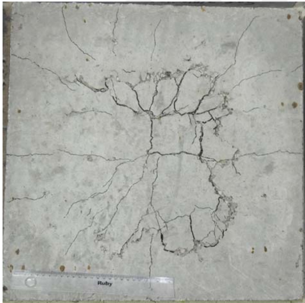
Specimen code; SF0.5 P_u = 71.44 \text{ kN} f'_c = 68.92 \text{ MPa} \rho = 1.1 \% V_f = 0.5 \% of SFRC
