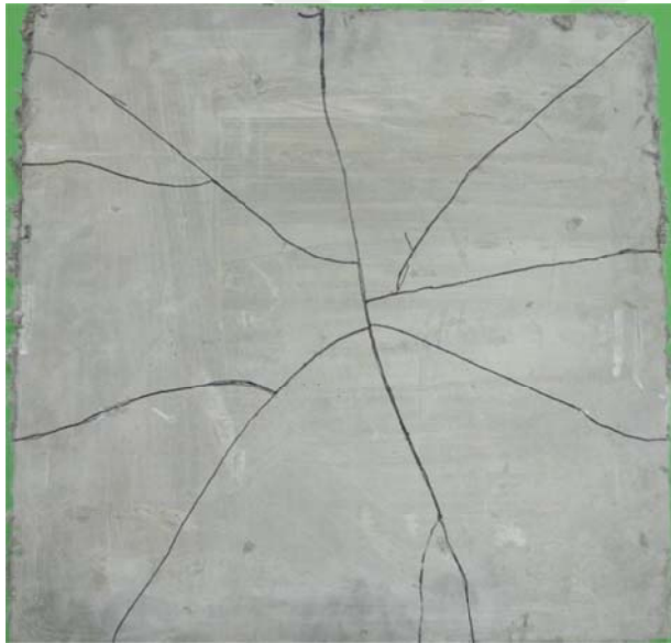
Specimen code; NM0.5 P_u = 13.7 \text{ kN} f'_c = 37.94 \text{ MPa} \rho = 0.0 \% V_f = 0.5 \% of NMECC
