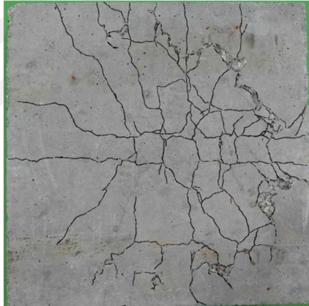
Specimen code; P60-11 P_u = 74.89 \text{ kN} f'_c = 43.20 \text{ MPa} h = 60 \text{ mm} Normal concrete
