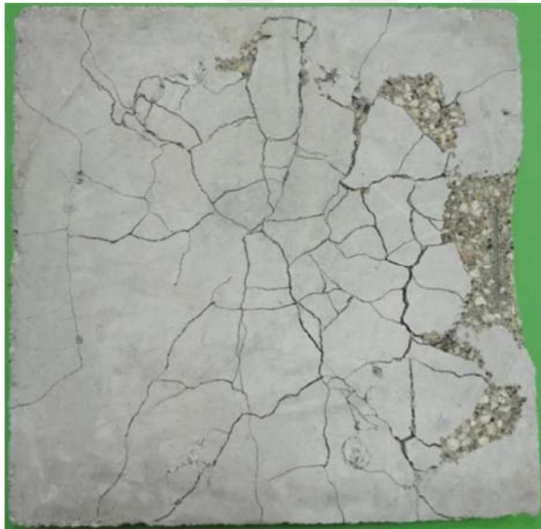
Specimen code; P60-10B P_u = 63.41 \text{ kN} f'_c = 40.83 \text{ MPa} \rho = 1.1 \% Normal concrete
