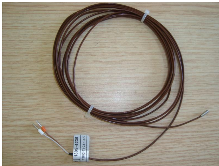
Figure 3.7 The used type T thermocouples
