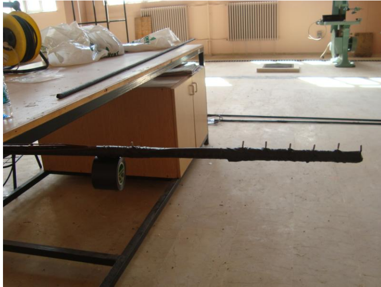
Figure 3.19 Covering of thermocouple wires with the second isolation layer
