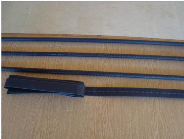
Figure 3.18 Covering the steel bars with the rubber tubes
