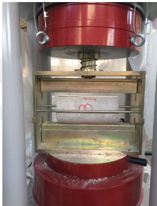
Figure 3.15 Splitting tensile test.
