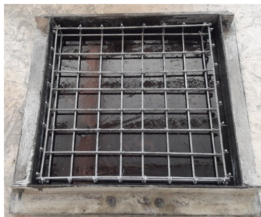
Figure 3.3 Casting mold and reinforcement details
