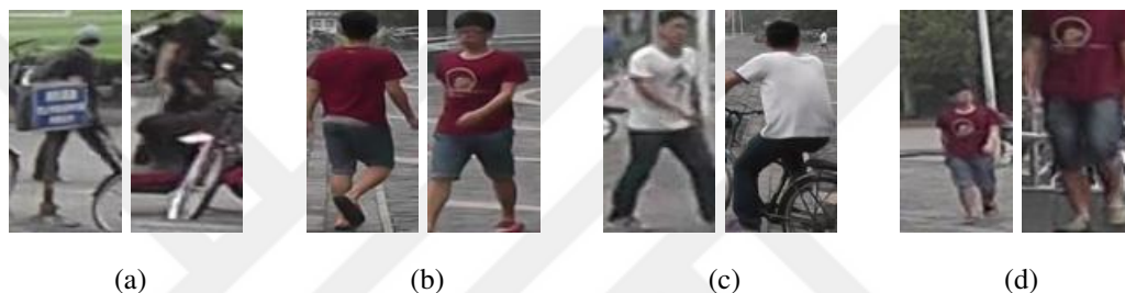
Figure 1.1: Some challenging examples from the Market-1501 dataset [1]. (a) Occlusion. The person-of-interest can be occluded by another object. (b) Viewpoint variation. The angle we are capturing the person may change. (c) Pose change. People can be in several poses. (d) Misalignment. Due to the errors of the detection algorithms, a person may not be aligned in the same way throughout their appearances.
