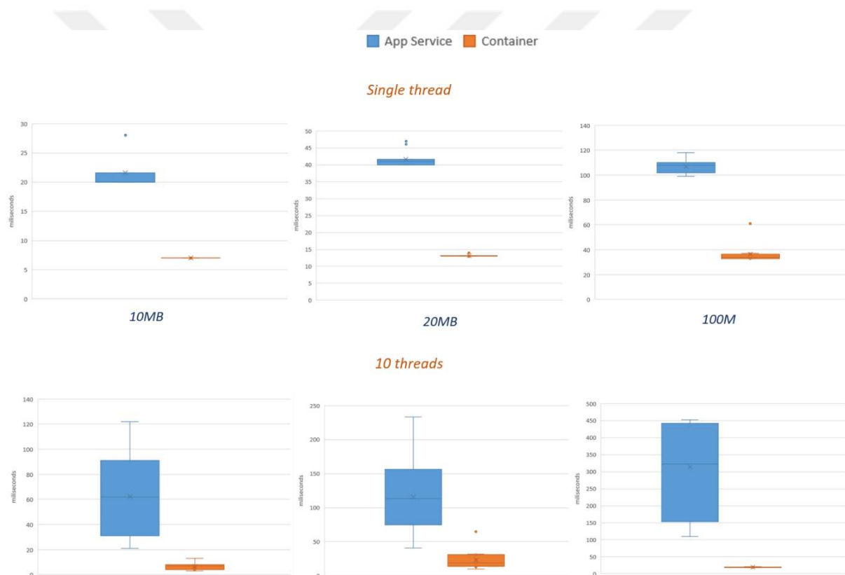
Figure 4.4 Memory read performance comparison between App Service and docker container in Azure
