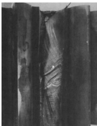
Figure 3.14 Tooth-bending fatigue from the root radius, loaded side, one-third from the open end.
