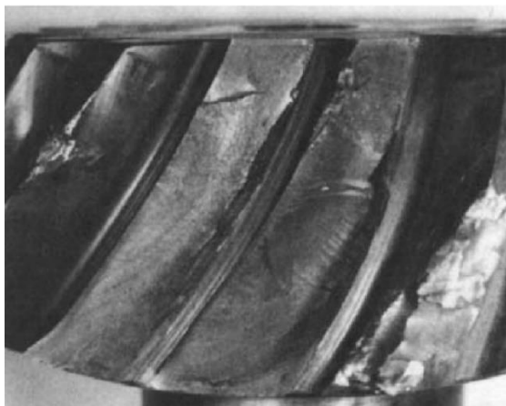
Figure 3.12 Spiral bevel pinion displaying the typical fatigue of the tooth bending.
