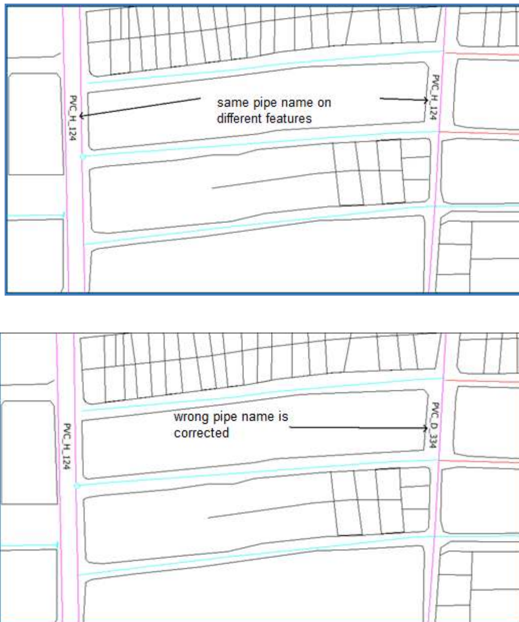
Figure 4.10 Wrong pipe names
