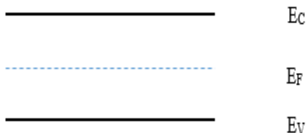
Figure 3.15. Natural diagram of semiconductor
