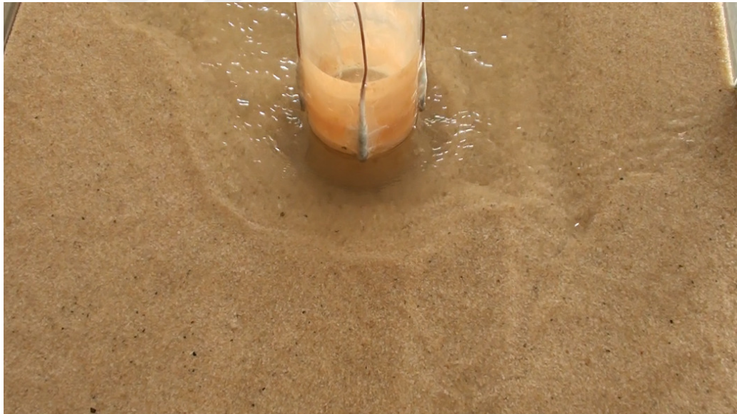
Figure 5.2 d) Scour hole of the D11 pier on Hid2020-44 at 40 mins (end) of the flood (Personal archive, 2018)
