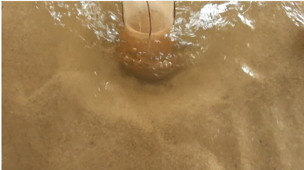
Figure 5.2 b) Scour hole of the D11 pier on Hid2020-44 at 20 mins (peak) of the flood (Personal archive, 2018)
