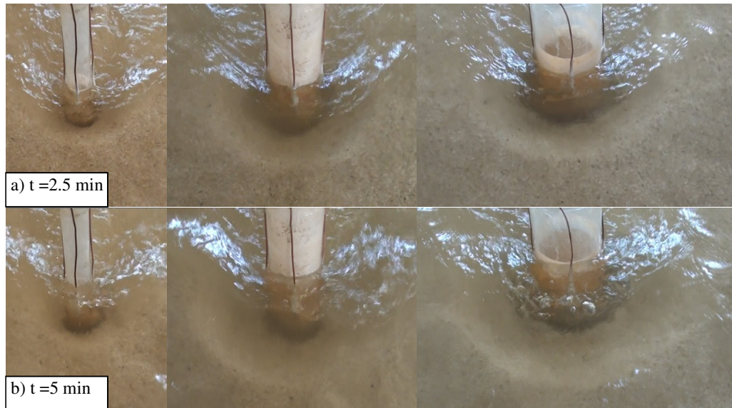
Figure 5.26 a, b, c and d) Sizes of the scour holes for different piers under Hid55-44 (Personal Archive, 2018)
