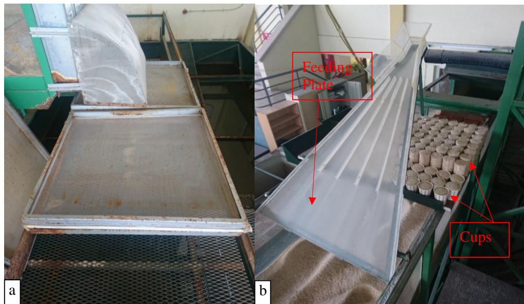
Figure 4.5 a) Sediment baskets b) Sediment feeding plate and cups (Personal archive, 2018)
