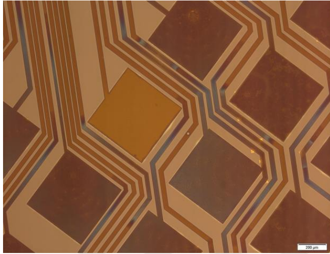
Figure 4.15: Defects on metals of electrical connection pads after wafer bonding process.
