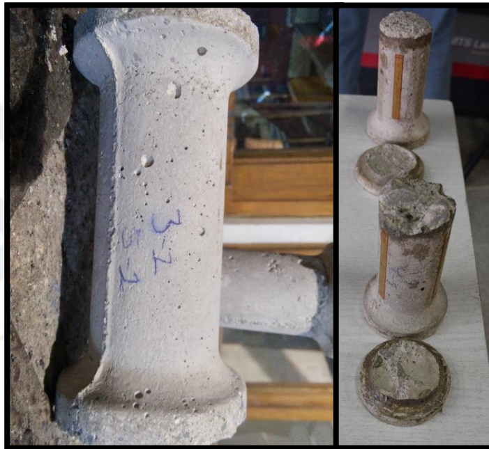
Figure 3-7 Dog-Bone Shaped Sample. Dimensions (a), Samples Photos Before and After the Test (b)
