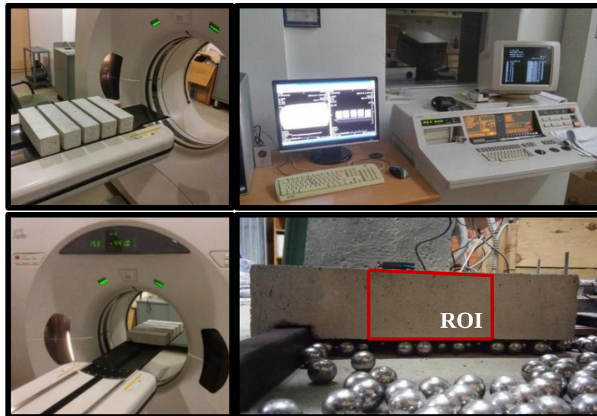
Figure 4-12 Scanning Concrete Samples via Tomography
