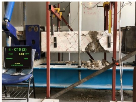
c) @ 13.3 kN.m.(moment) vs 133.0 \times 10^{-3} rad/m (twist)
