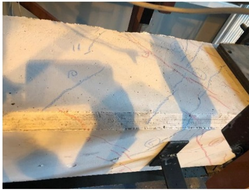
a) @ -12.1 kN.m.(moment) vs -5 \times 10^{-3} rad/m (twist)
