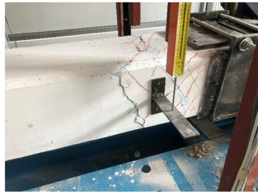
b) @ -14.0 kN.m (moment) vs -5.3 \times 10^{-3} rad/m (twist)
