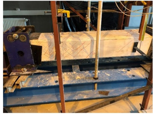
b) @ -28.9 kNm (moment) vs -13.4 \times 10^{-3} rad/m (twist)
