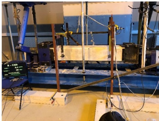
a) @ 26.0 kN.m.(moment) vs 3.1 \times 10^{-3} rad/m (twist)
