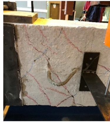
b) @ 15.6 kN.m.(moment) vs 12 \times 10^{-3} rad/m (twist)
