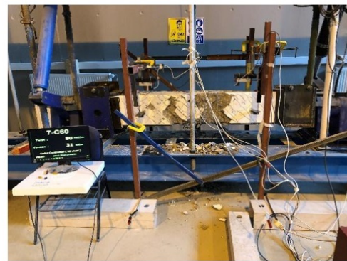
d) @ 31.0 kN.m.(moment) vs 80.0 \times 10^{-3} rad/m (twist)
