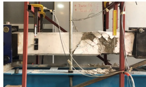
b) @ 15.6 kN.m.(moment) vs 12 \times 10^{-3} rad/m (twist)
