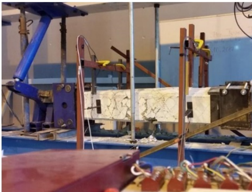
c) @ 13.3 kN.m.(moment) vs 130.4 \times 10^{-3} rad/m (twist)
