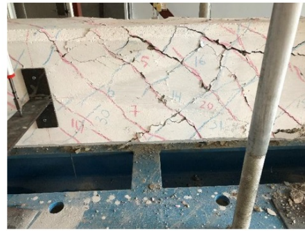
b) @ 15.6 kN.m.(moment) vs 95.2 \times 10^{-3} rad/m (twist)
