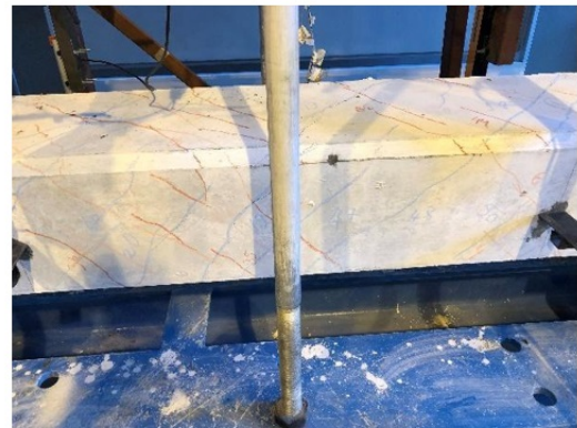
b) @ -23.9 kN.m.(moment) vs -20.0 \times 10^{-3} rad/m (twist)
