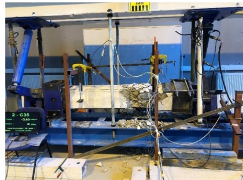
d) @ -8.7 kN.m (moment) vs - 210.0 \times 10^{-3} rad/m (twist)
