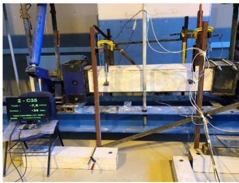
a) @ -24.0 kN.m (moment) vs - 7.5 \times 10^{-3} rad/m (twist)
