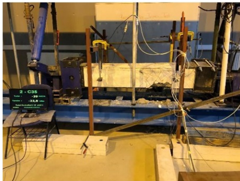
c) @ -22.8 kN.m (moment) vs - 39.0 \times 10^{-3} rad/m (twist)
