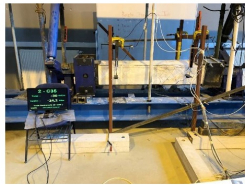
b) @ -24.2 kN.m (moment) vs - 30.0 \times 10^{-3} rad/m (twist)
