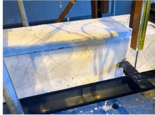
b) @ -24.0 kN.m (moment) vs - 12.0 \times 10^{-3} rad/m (twist)
