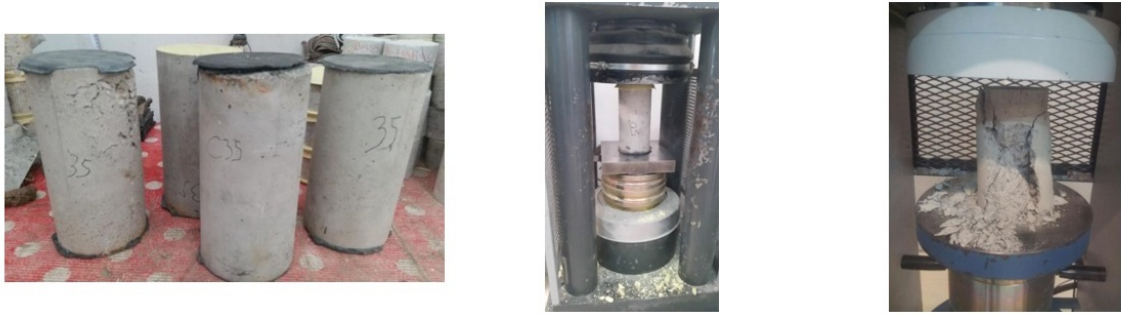
Figure 4.4. Testing of concrete samples.
