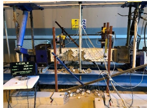
d) @ 26.6 kN.m (moment) vs 120.0 \times 10^{-3} rad/m (twist)
