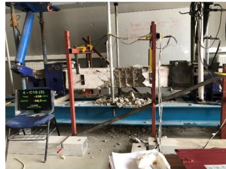
d) @ -10.3 kN.m.(moment) vs -228.0 \times 10^{-3} rad/m (twist)
