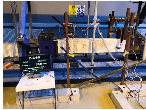
b) @ 25.8 kN.m.(moment) vs 12.0 \times 10^{-3} rad/m (twist)
