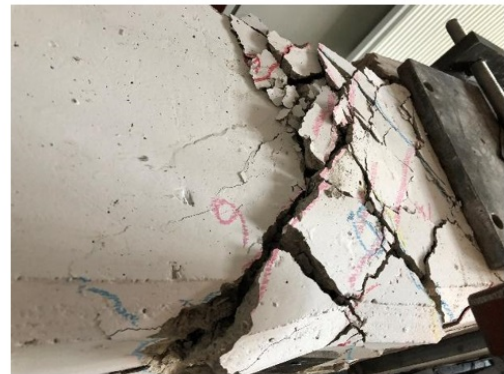
d) @ -15.3 kN.m (moment) vs -12.6 \times 10^{-3} rad/m (twist)
