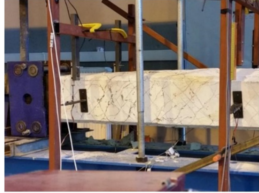
b) @ 15.7 kN.m.(moment) vs 95.2 \times 10^{-3} rad/m (twist)
