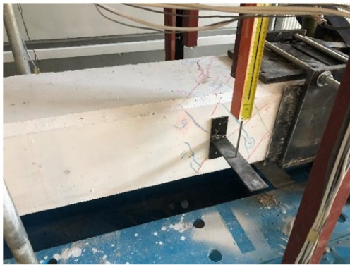
a) @ -14.7 kN.m (moment) vs -3.2 \times 10^{-3} rad/m (twist)
