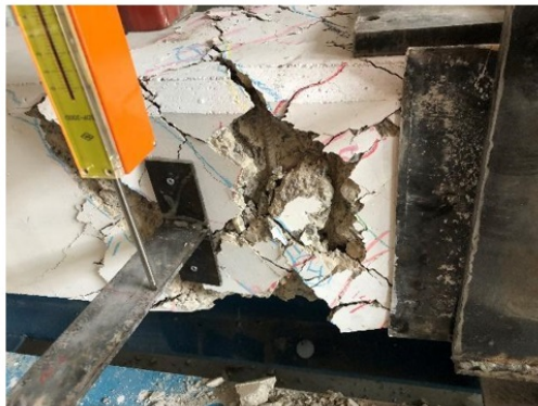
c) @ -14.6 kN.m (moment) vs -10.5 \times 10^{-3} rad/m (twist)
