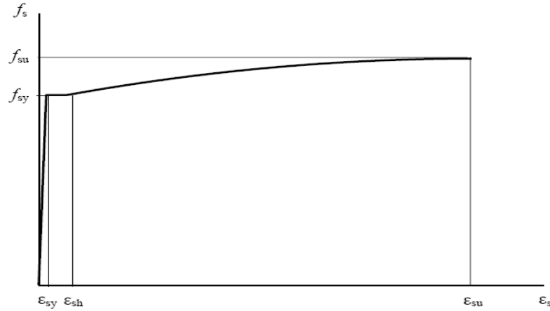
Figure 2.8 : Stress-strain relation for steel reinforcement. (DBYBHY 2007)
