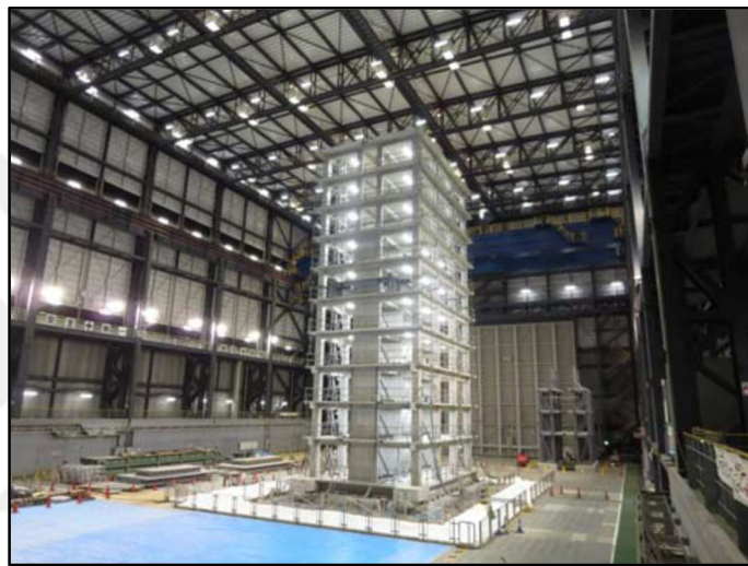
Figure 4.4. Photograph of 2015 E-defense 10-story building specimen.
