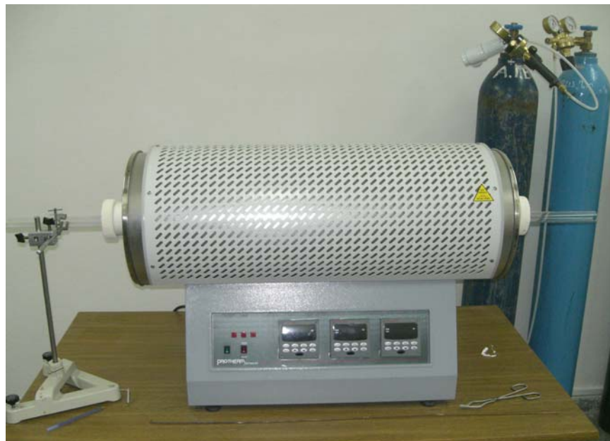
Figure 5.5: PROTHERM (Model PTF 12/75/200) programmable tube furnace.
