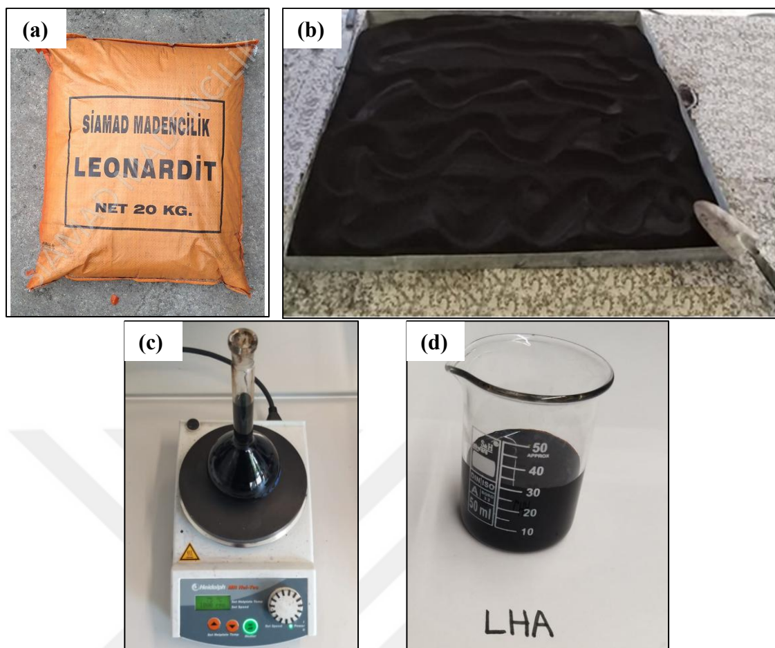
Figure 3.3 (a) Leonardite raw material, (b) Ground leonardite, (c) LHA production process, (d) Final product LHA
