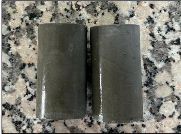
Figure 3.7 Cylindrical compressive strength test samples
