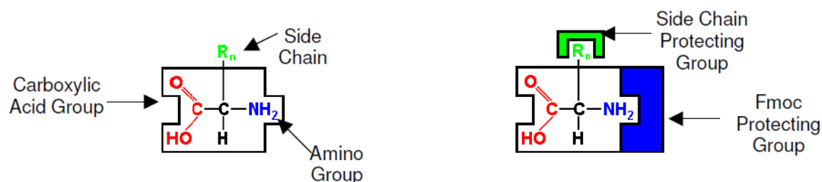
Figure 3.3: In order to conjugate one amino acid at a time, amino and the reactive side chain groups must be protected. As the peptide grows from C to N direction, carboxyl group must be activated. This figure shows the difference of the amino acid which will be used in SPPS. Adapted from [58].
