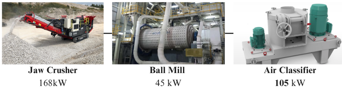
Figure 3.6: Brick Repurposing Production Line and Electric Consumptions
