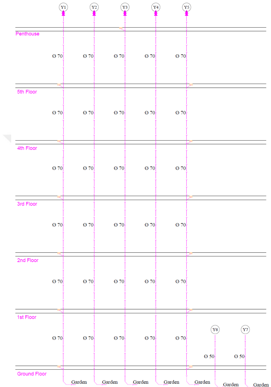
Figure A.15 Storm Water Piping System
