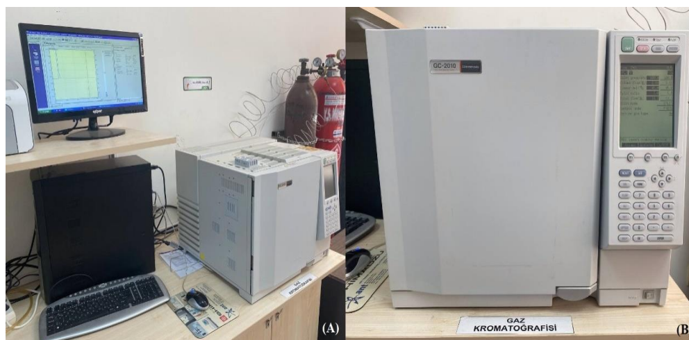
Figure 3.3 Gas chromatography (Shimadzu GC2010).
