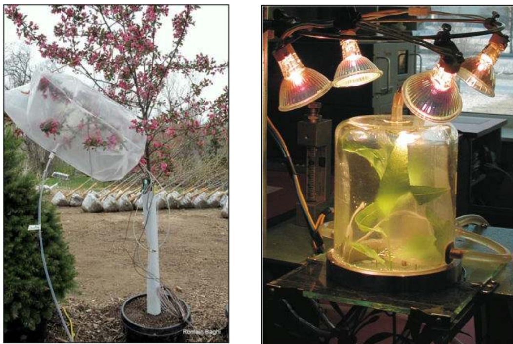
Figure 2.4 BVOC measurements in field and laboratory (Copolovici & Niinemets, 2010; Baghi et al., 2012).
