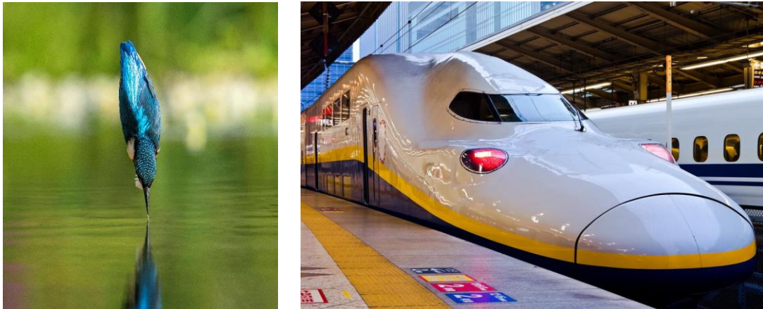
Figure 9: The Nose of the Bullet Train, Inspired from a Kingfisher's Beak (Primrose, 2020).
