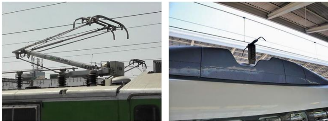
Figure 10: Pantograph in Conventional Trains (left) and Pantograph in Bullet Trains (right). Source: (Primrose, 2020).
