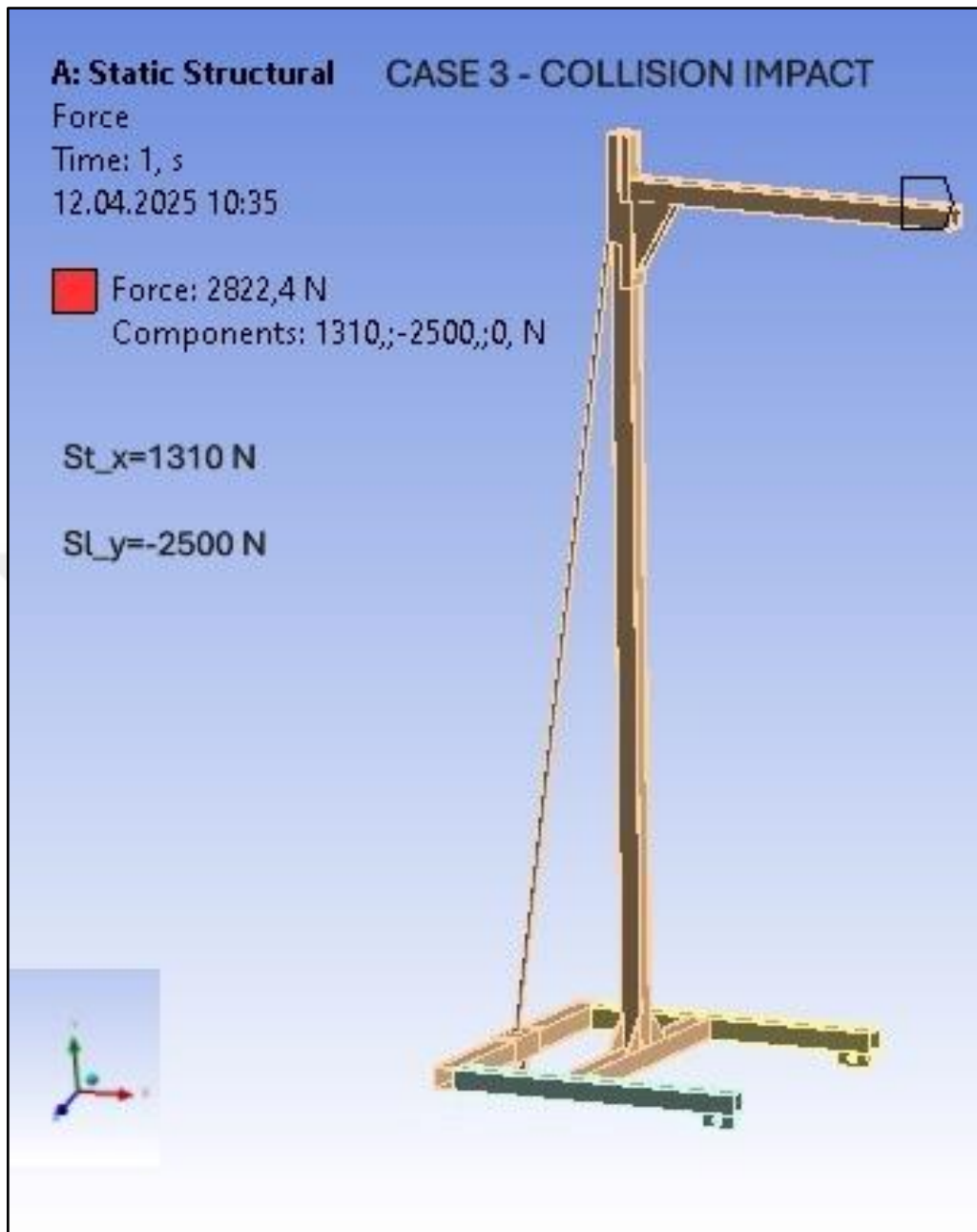
Figure 4.11: Forces. Case 3-Collision Loading.
