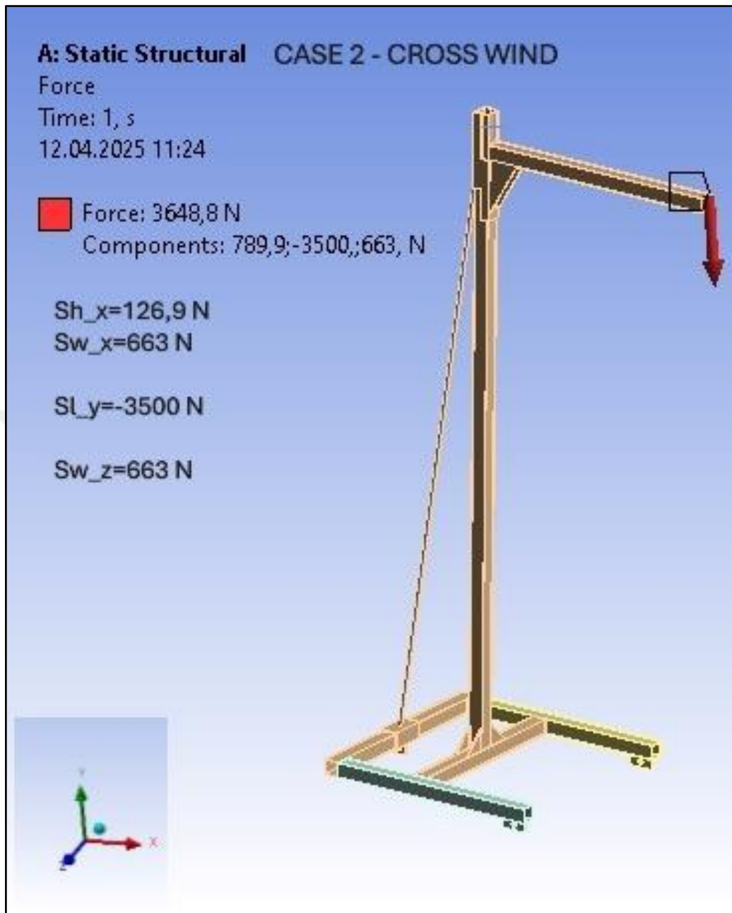
Figure 4.7: Forces. Case 2-Cross Wind Loading.
