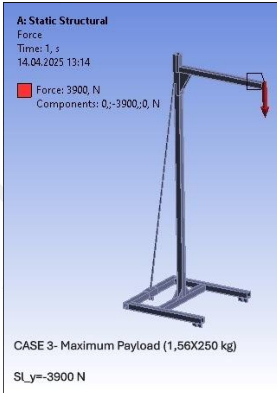
Figure 4.15: Forces. Case 3-Maximum Payload Loading.
