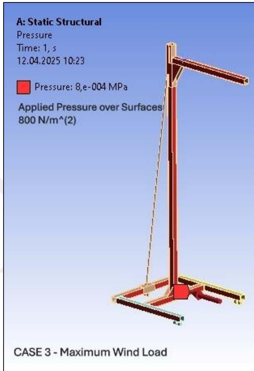
Figure 4.13: Maximum Wind Pressure on Surfaces. Case 3-Maximum Wind Loading.
