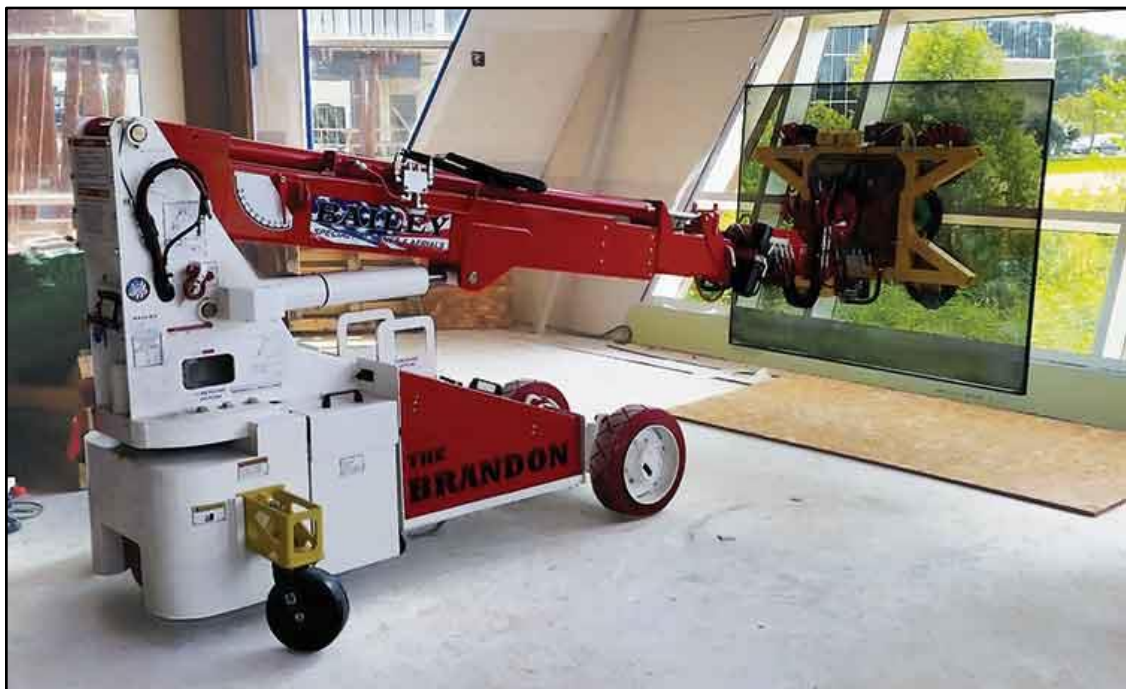
Figure 1.10: BRANDON 6 Mini Glass Lifter. 24 V Battery Powered [6].
