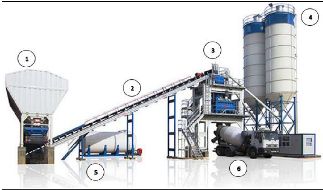
Figure 2.2 Components of a Batch Plant: Raw Material Bunker (1), Conveyor Belt (2), Mixer (3), Silos (4), Water Tank (5), and Truck-Mixer (6) (Mphahlele, 2017)
