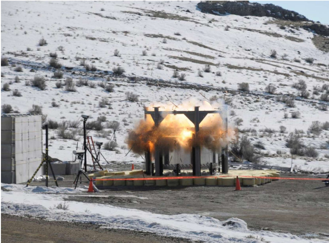
Figure 1-9. A full-scale separation test of the forward skirt extension for the Ares I-X[34]
