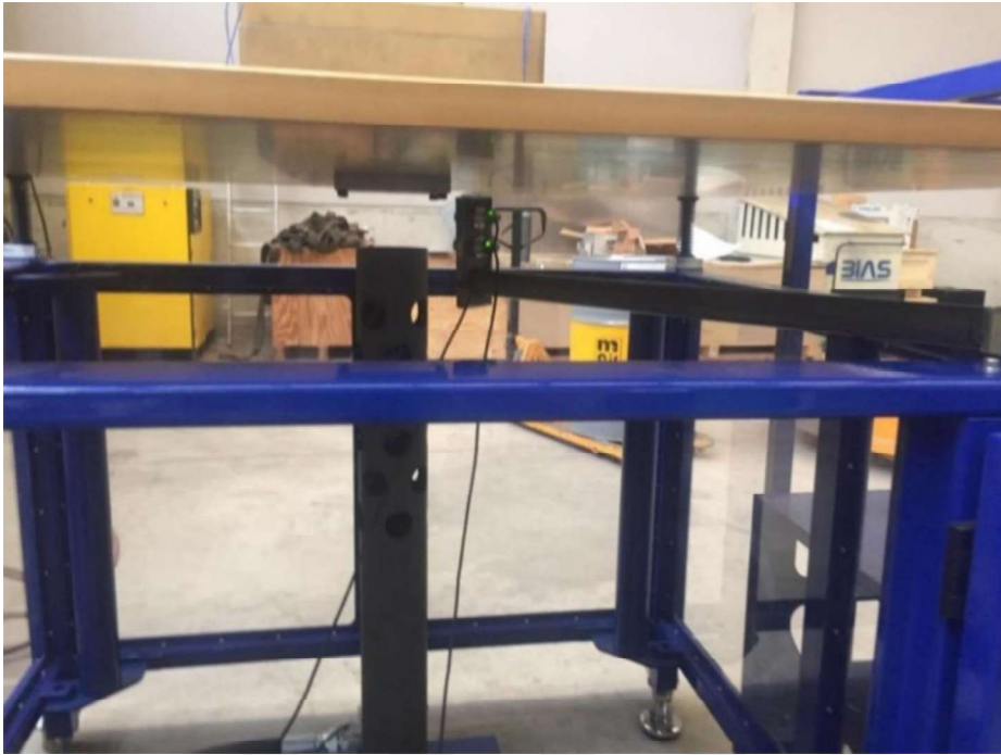
Figure 3-1. Laser sensors for velocity measurement
