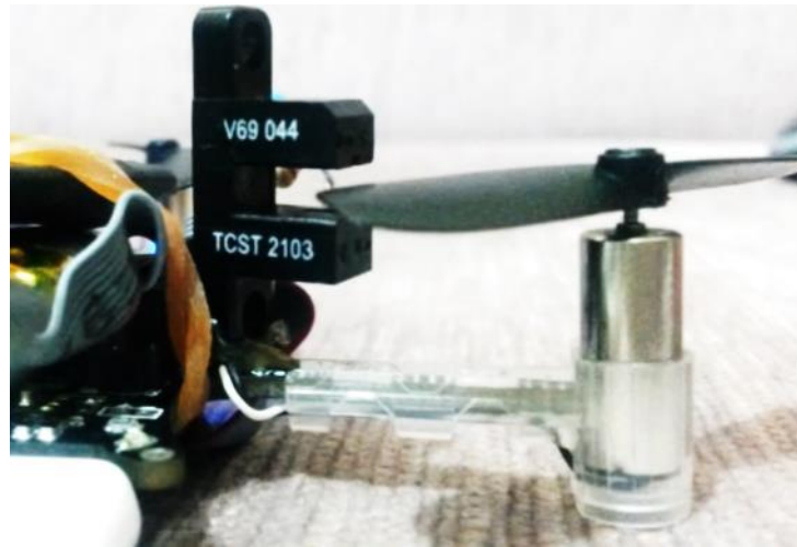
Figure 5.5 : Motor speed sensor.
