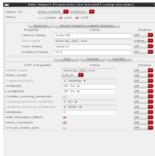
Figure 6.1: There are three effective parameters: length, width and the number of parallel of same capacitor which is named multiplier.
