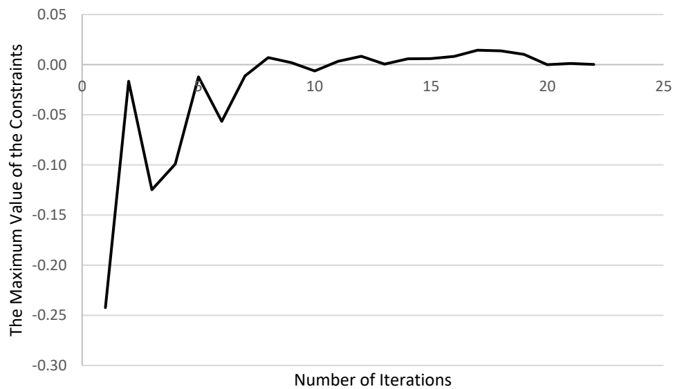
Figure 8-18 The Maximum Value of the Constraints vs Number of Iterations for Wing v2_1
