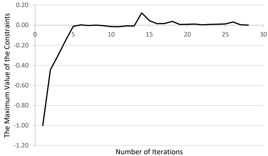
Figure 7-14 The Maximum Value of the Constraints vs Number of Iterations with Starting from the Maximum Design Variables
