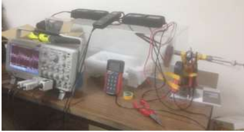
Fig. 5. The setup of the constructed wind energy harvester and wind tunnel.
