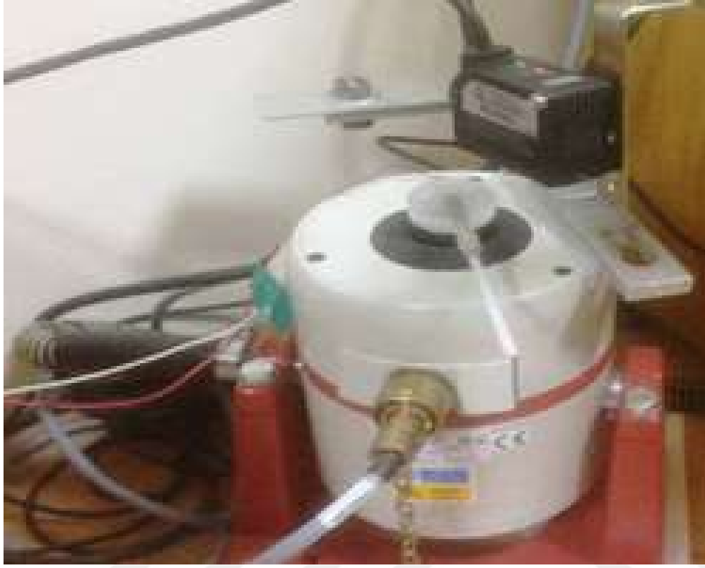
Fig. 3. The frequency response test of the piezoelectric layer by a shaker.
