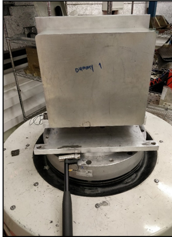
Figure 5.44. Hammer test setup and hammer hit locations
