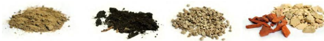
Figure 3.21 Examples of components in a growing medium. From left to right, sand, compost, pumice-stone and crushed brick
