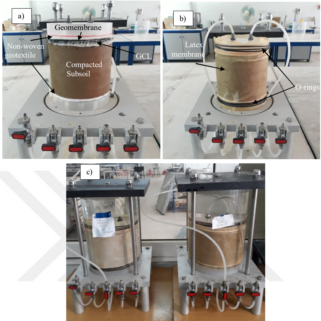
Figure 2.9 Sample preparation for the hydration of GCL: a) components, b) placement of latex membrane and O-rings, c) general view of permeameters during hydration (Personal archive, 2019)
