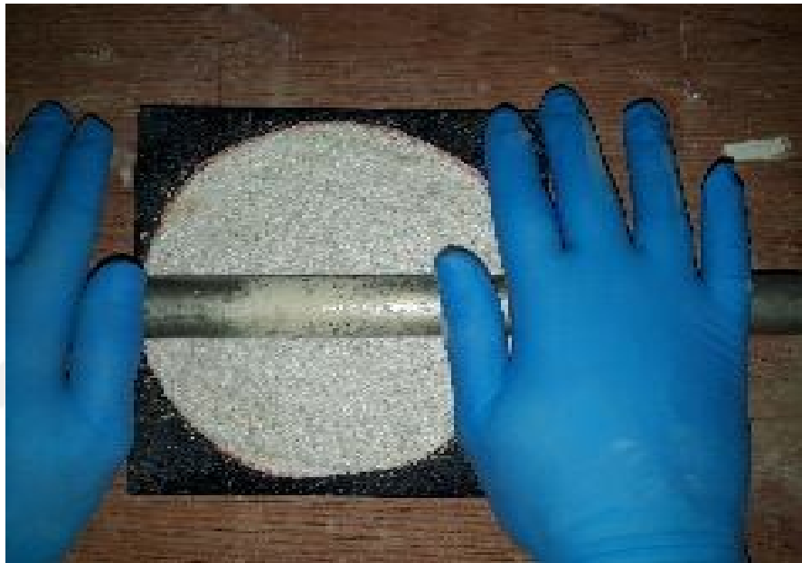
Figure 2.7 Arranging the mass per unit area (MPUA) of bentonite in GCL (Personal archive, 2019)
