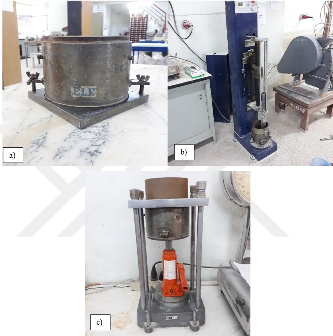
Figure 2.8 Photographs of compaction mold and compaction process: a) Compaction mold, b) compaction of subsoil by using automatic compactor and c) extrusion of compacted subsoil from mold (Personal archive, 2019)
