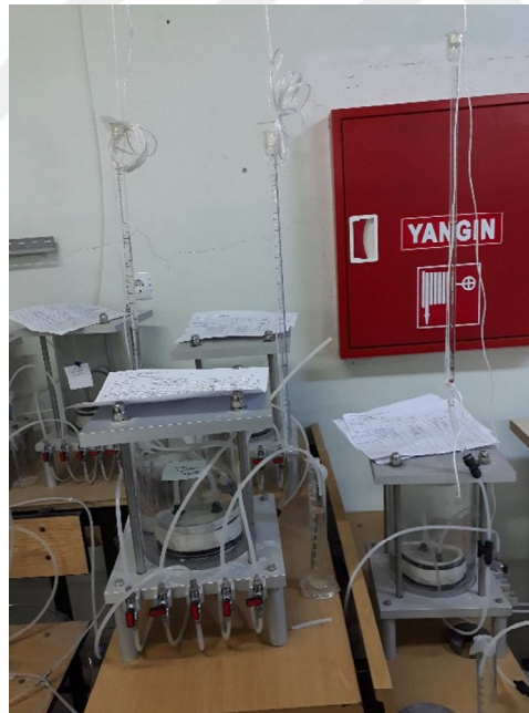
Figure 5.1 Overall view of the hydraulic conductivity tests under elevated hydraulic gradient (Personal archive, 2019)
