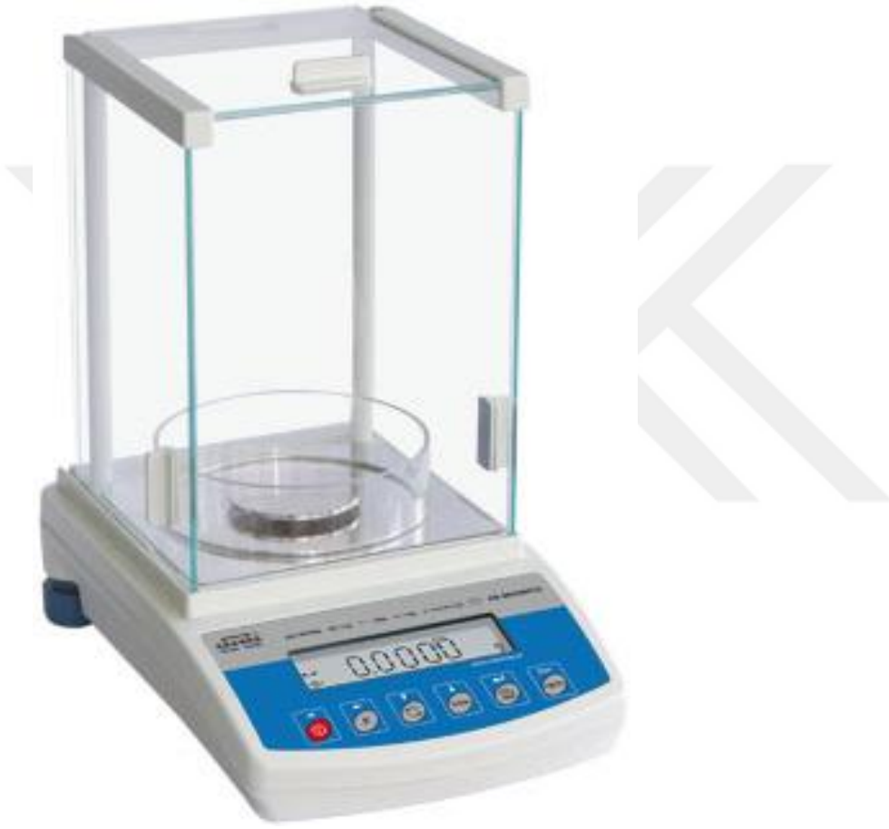
Şekil 4.2. Radwag AS 220/C/2 hassas terazi
