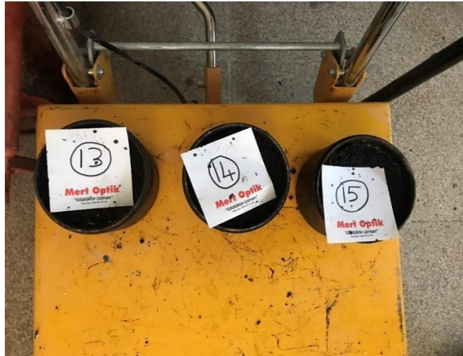
Figure 4.2 Compacted specimens of AASHTO R30 method after short term conditioning (Personal archive, 2019)
