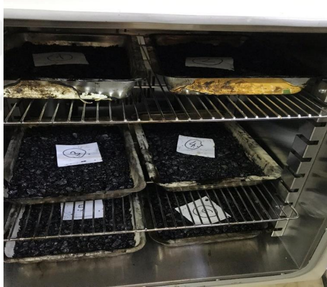
Figure 4.1 Short term conditioning of AASHTO R30 method in a forced-draft oven (Personal archive, 2019)
