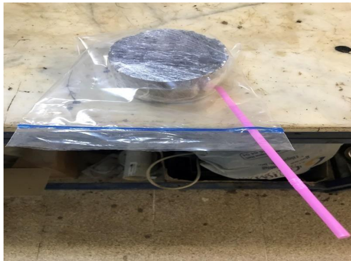
Figure 4.10 Vacuuming the specimen and putting it in a heavy duty leak-proof plastic (Personal archive, 2019)
