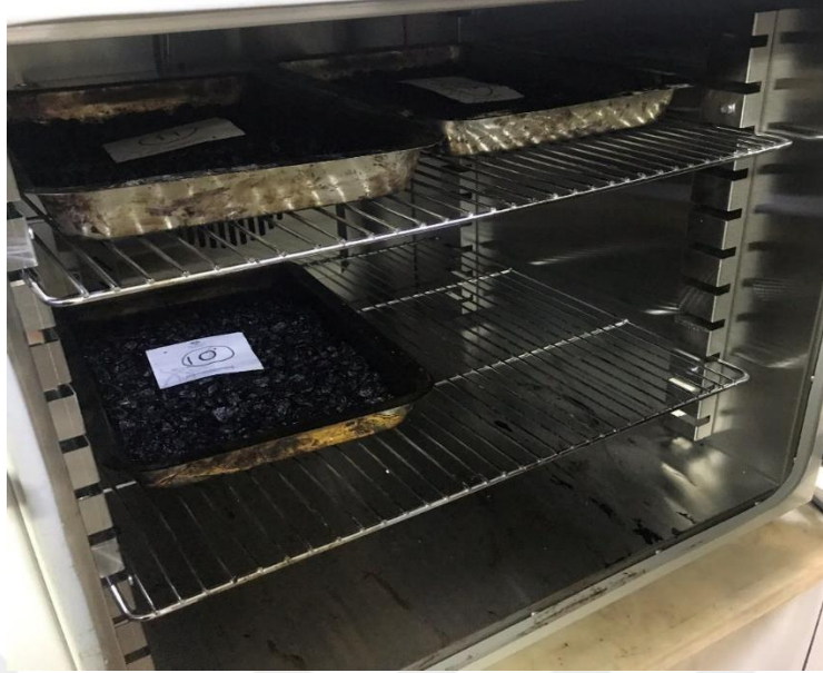
Figure 4.5 Short term conditioning of RILEM method (Personal archive, 2019)
