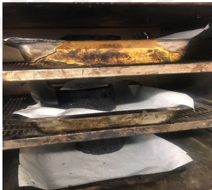
Figure 4.3 Long term conditioning of AASHTO R30 method in a forced-draft oven (Personal archive, 2019)
