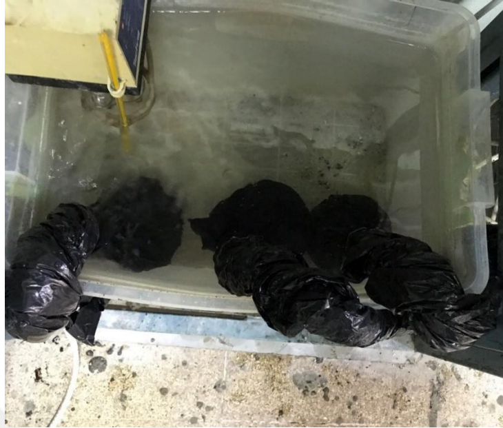
Figure 4.11 Water bath at 25 °C (Personal archive, 2019)
