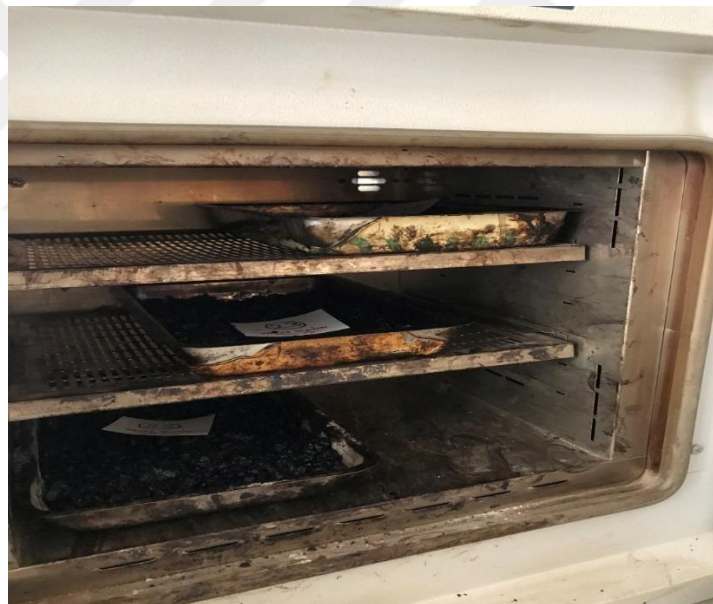
Figure 4.6 Long term conditioning of RILEM method (Personal archive, 2019)
