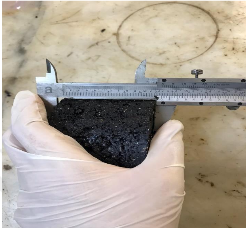
Figure 4.8 Asphalt height measurement with caliper (Personal archive, 2019)
