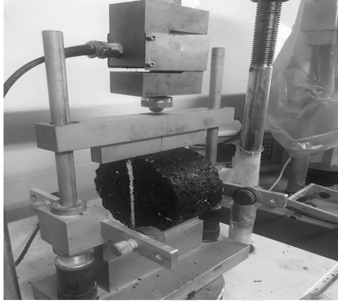
Figure 4.12 A true assemble of specimen for ITS test (Personal archive, 2019)
