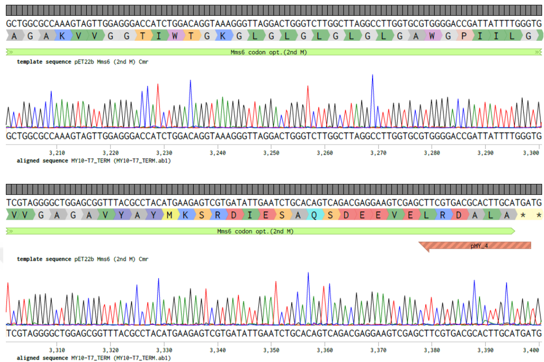
Figure D 1. Sanger DNA sequence verification results for pET22b 6H Mms6 cloning.
