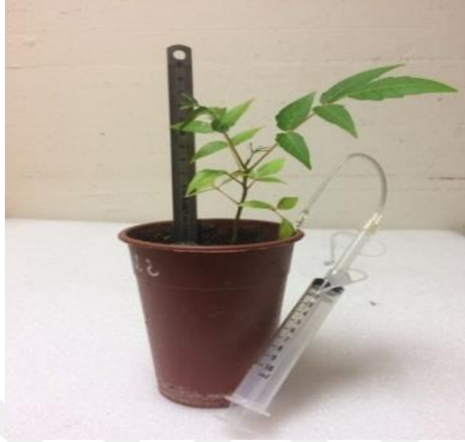
Şekil 3.13: Toprak gözenek suyu analizi (Rhizon®, model MOM, Rhizosphere Research Products, Wageningen, Netherlands).
