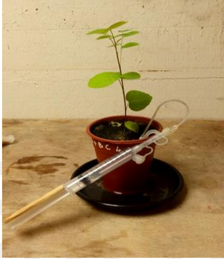
Şekil 3.21: Gözenek suyu analizinden bir kesit (Rhizon®, model MOM, Rhizosphere Research Products, Wageningen, Netherlands).
