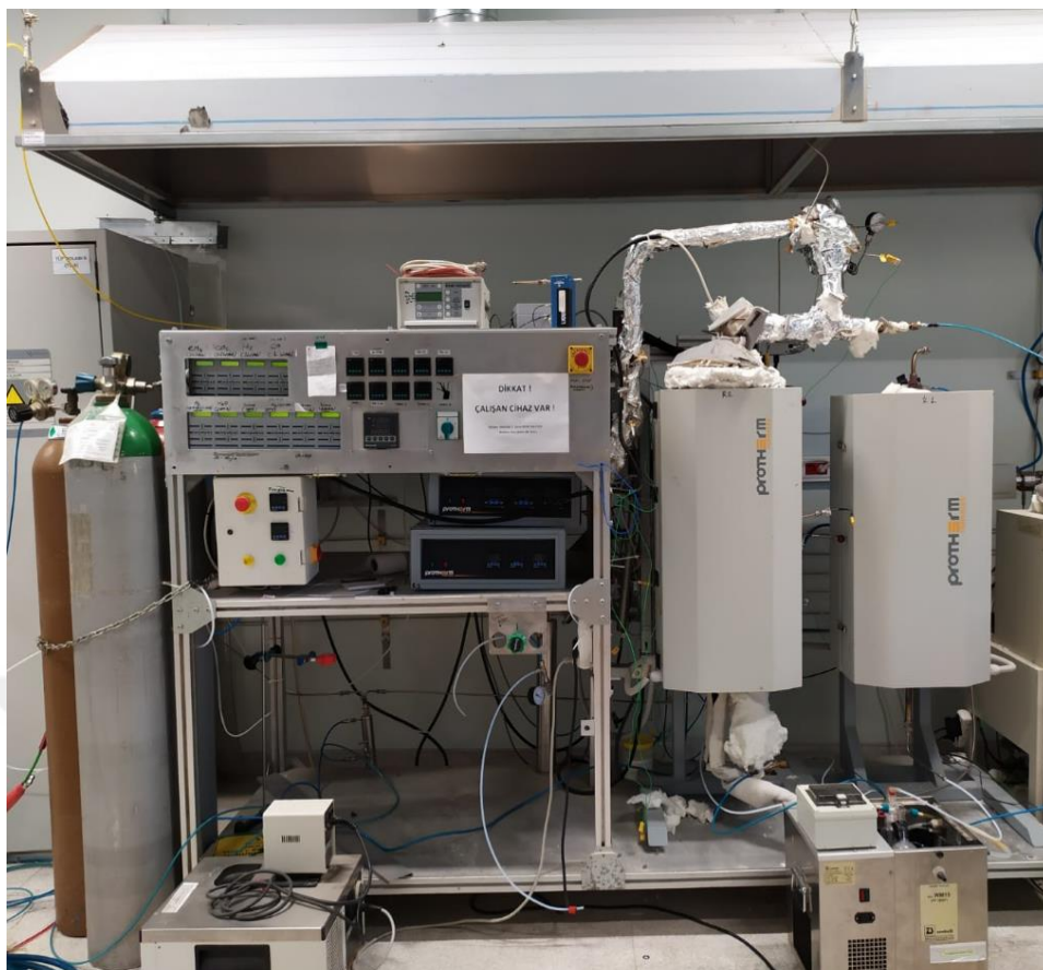
Figure 4.5: Experimental set-up for H 2 S adsorption
