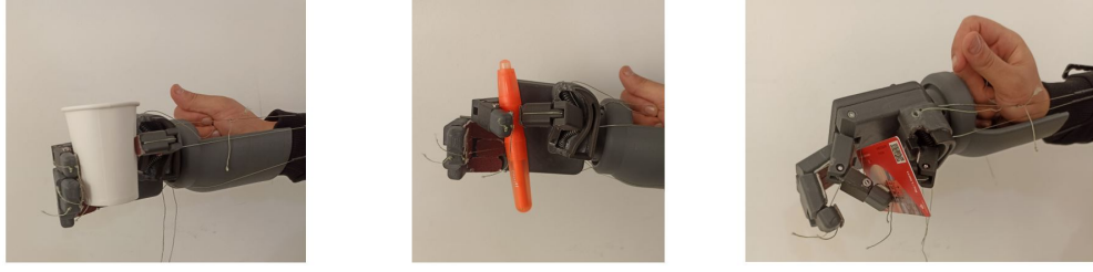
Figure 7: Multi-size object handling with HandMech: paper-cup(left), pen (middle), and card (right)
