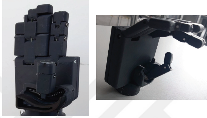
Figure 5: Prototype of the hand prosthesis: the fully open posture (Left), and the natural posture (Right)
