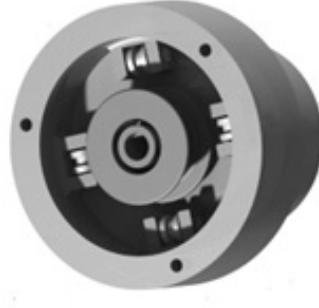
Figure 11: Assembly of pulleys inside the wrist base part
