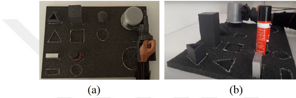
Figure 9: SHAP test for body-powered hand prosthesis: top view (a), side view (b)
