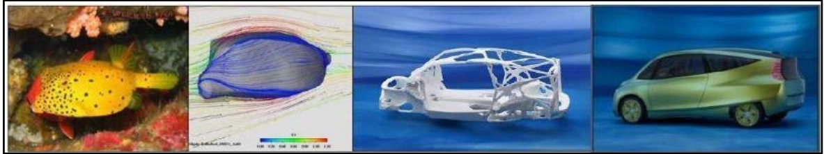
Figure 2.9. Design of the bionic car by Daimler Chrysler [25].
