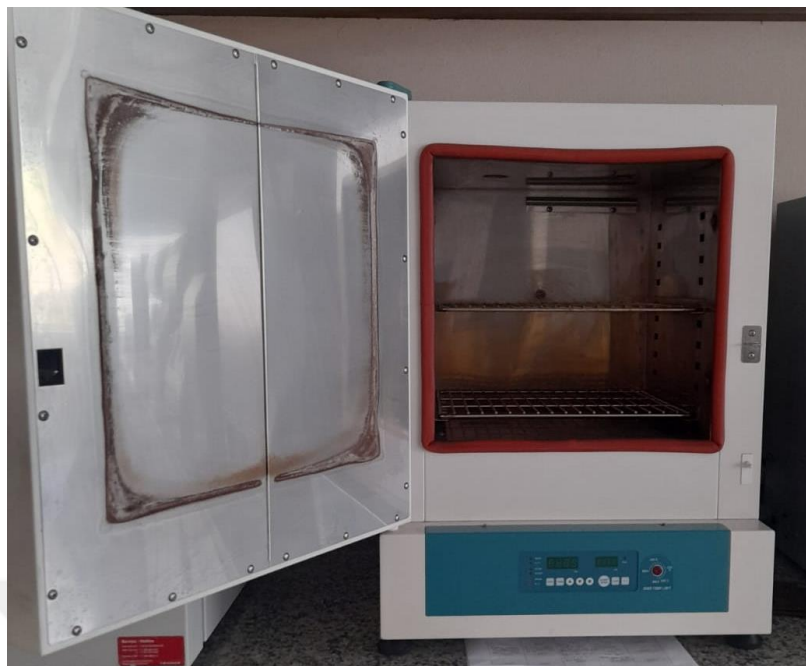
Figure 4.3 Oven used in the preparation of catalyst supported substrates to be sent to the CVD system.
