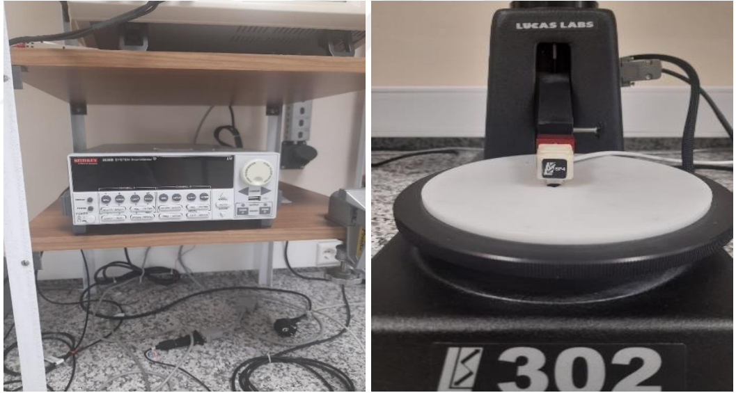
Figure 4.14 Current-Voltage Characterization Device, Keithley 4200 analyzer (Electric-Electronic Measurement Lab., DEU).
