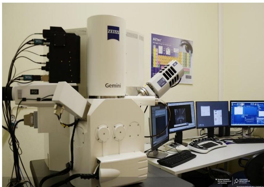
Figure 4.9 Device used in EDX characterization, Carl Zeiss Sigma 500-FESEM (Optical Imaging Lab., IBG)
