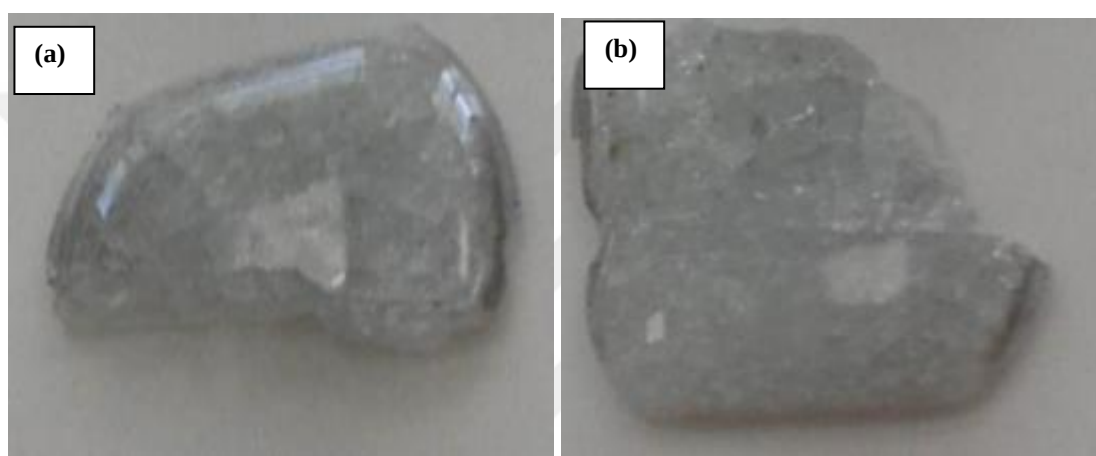
Figure 5.3 Images of samples 7 and 8 after CVD process at 1000°C; (a) Sample 7, (b) Sample 8
