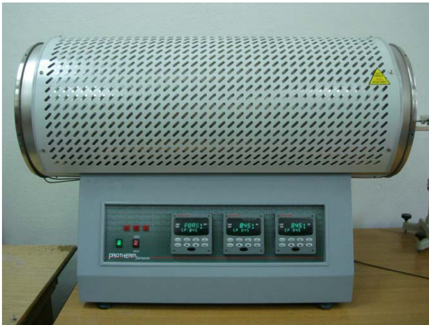
Figure 3-7: Protherm PZF 12/75/700 Three Zone Tube Furnace
