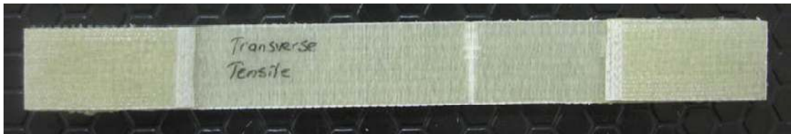
Figure 5. Deformed tensile test specimens to obtain transverse elasticity module ( E_2 ) and transverse tensile strength ( Y_t )
