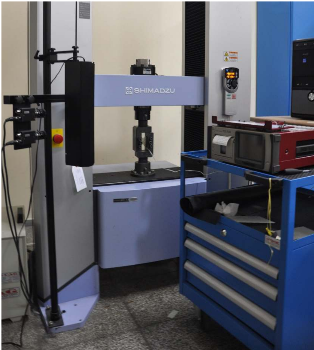
Figure 3.14 Connected indicators to the specimen in V-notched rail shear test process
