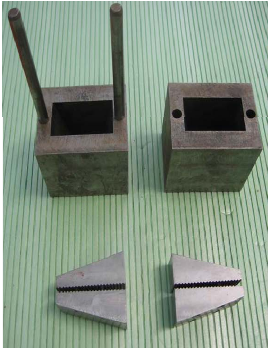
Figure 3.6 A view of compression testing equipment
