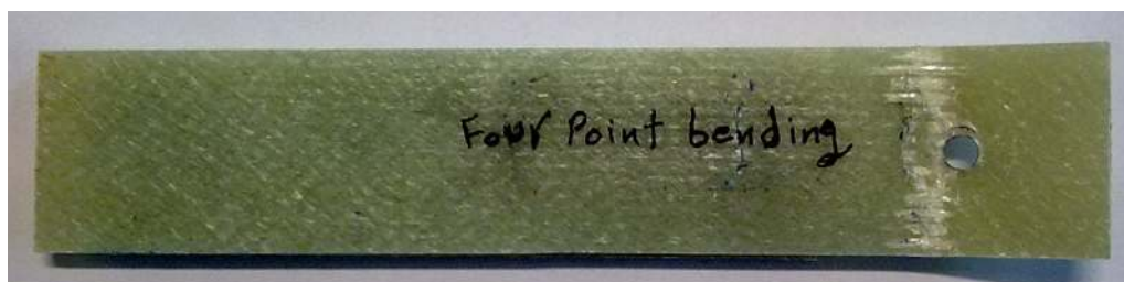
Figure 5.5 The failure mode's photograph of tested specimen at four point bending moment
