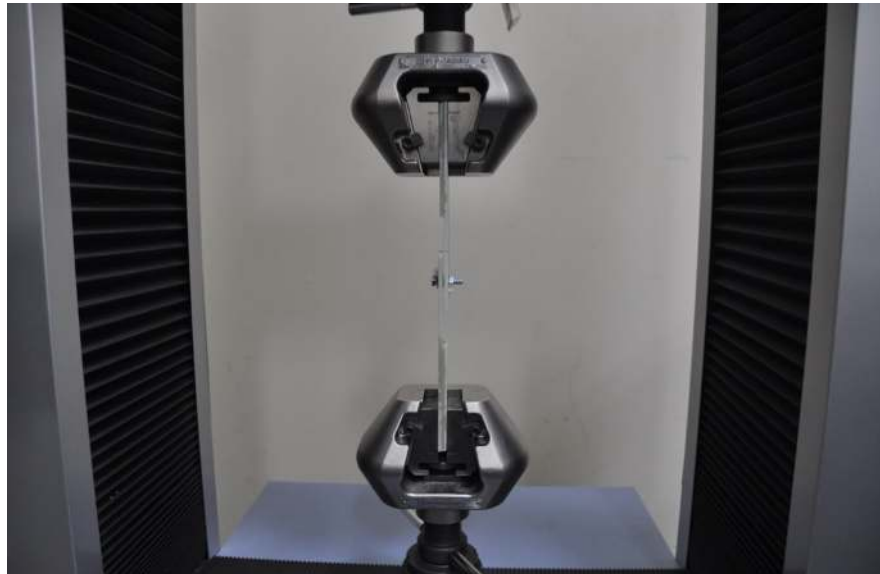
Figure 4.4 bolt loaded glass-epoxy laminated composite test process
