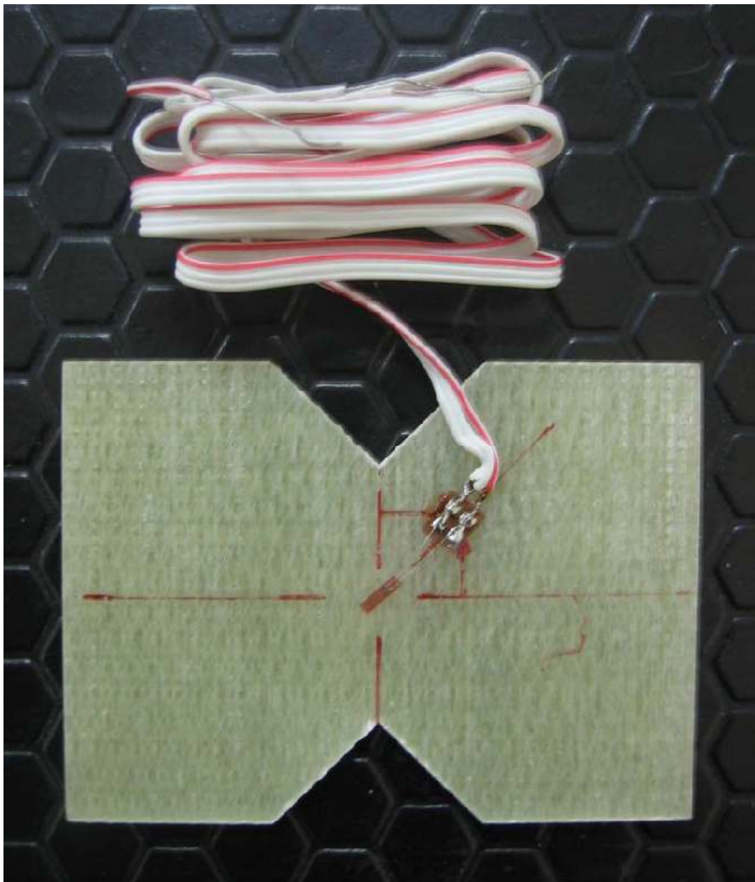
Figure 3.11 V-notched rail shear test specimen before tested.
