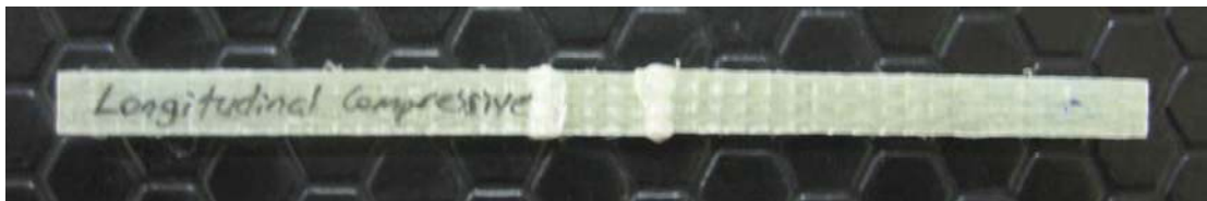
Figure . Deformed longitudinal compressive test specimens to obtain longitudinal compressive strength ( X_c )
