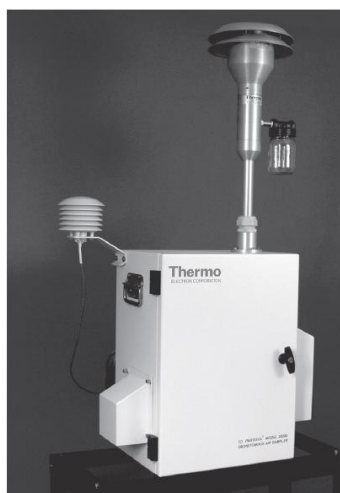
Figure 2.2. Thermo rp Partisol 2000-D dichotomous sampler
