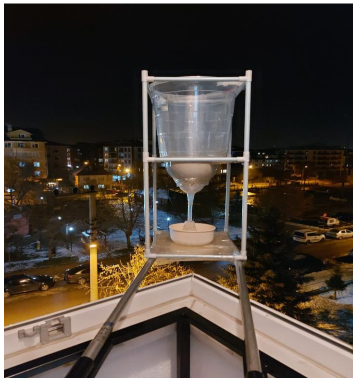
Picture 3.1. Manual system for collection of rainwater samples
