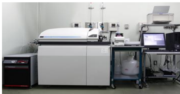
Picture 3.3. A photo of the Perkin-Elmer ELAN DRC-e model ICP-MS system in the laboratory
