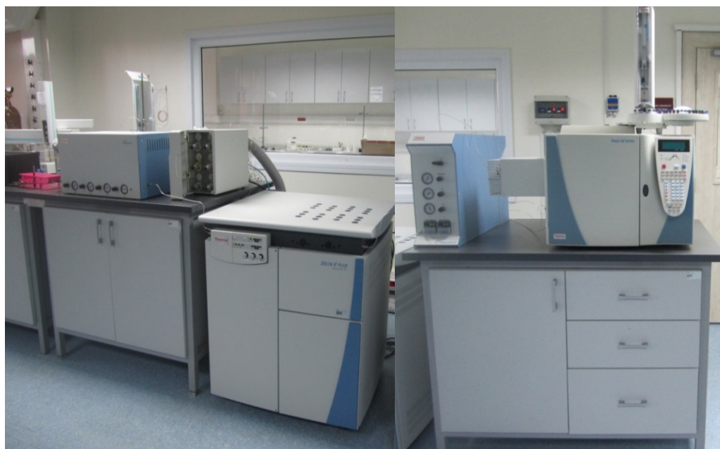
Figure 4.8. EA-IRMS instrument used in the analysis of collected samples
