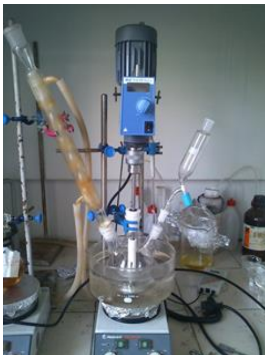
Figure 2.1: Resin synthesis set-up.
