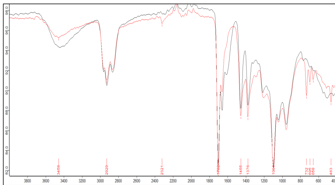
Figure 3.32: FTIR spectra of MEKFR-BA and MEKFR.
