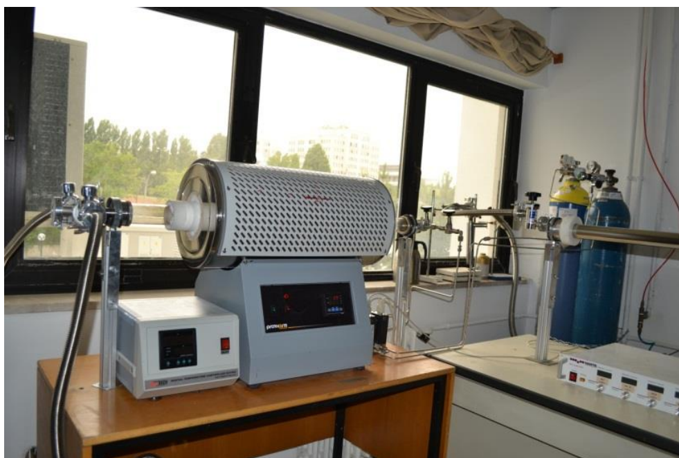
Figure 11. Chemical vapor deposition system for the production of BNNTS (real picture)
