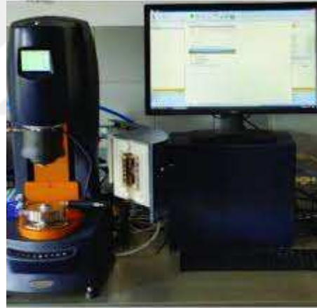
Şekil 3.11. TA marka DHR-1 model Discovery Hybrid Reometer-1
