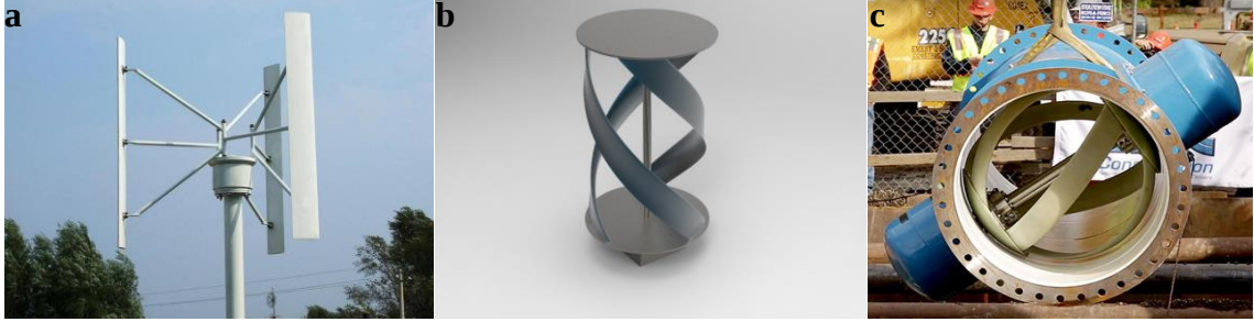
Şekil 10.(a) Darrieus türbini (Wu ve ark., 2014), (b) Gorlov sarmal türbin (Swik, 2019), (c) Lucid Küresel Türbini (Hopman, 2017)
